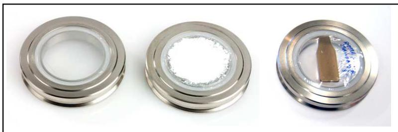
Fig. 5: Typical sample preparations between thin mylar foils: left – empty sample holder for a background measurement, middle – nanopowder sample, right – polymer nanocomposite.
