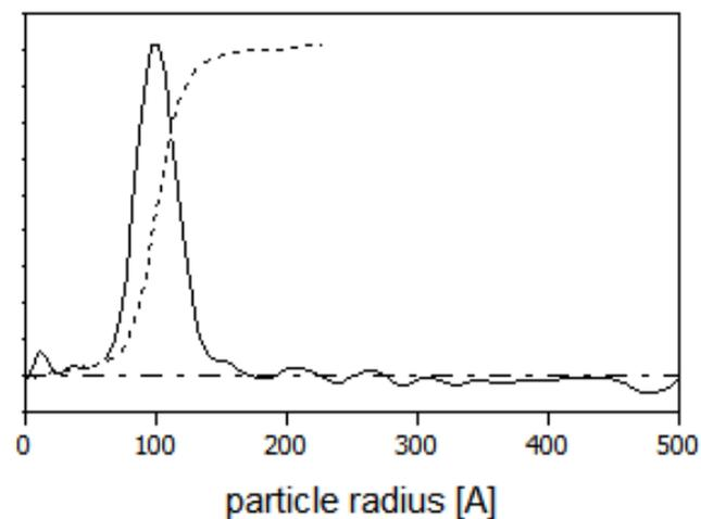
Figure 2. Volume-weighted particle size distribution  $D_V(r)$  for aqueous dispersion of FD100 shows a well-defined single-mode distribution. Particle radius is shown as abscissa.
