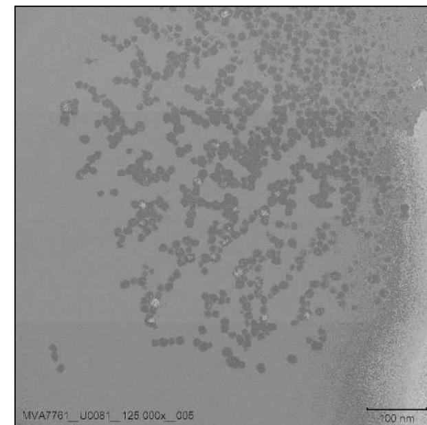
*Figure 1. A mono-modal particle population with a modal diameter of 180 [Å] estimated with number-weighted particle size distributions by TEM.<sup>[2]</sup>*
