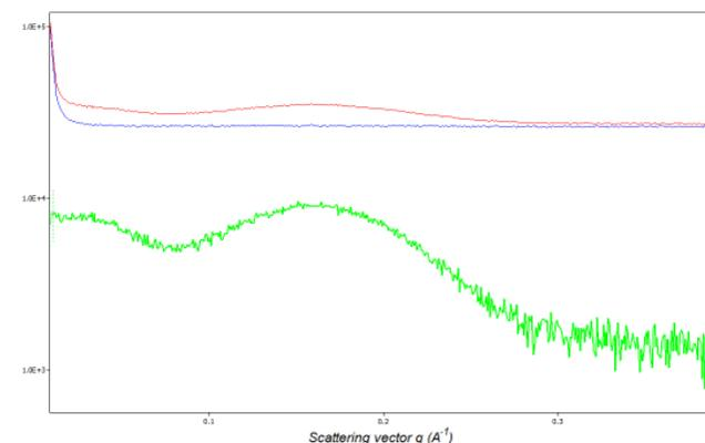
Figure 1. SAXS pattern of SDS dispersion is shown in red, pattern of water is shown in blue and their differential is shown in green.
