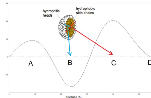
Figure 2. Minimum and maximums of the reconstructed PDDF function indicate the characteristic distances within the particle.
