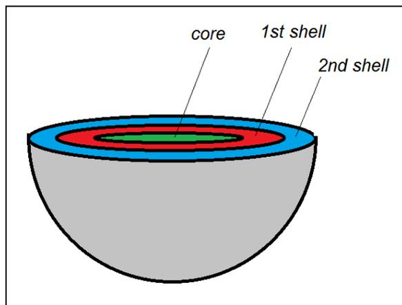
Figure 3. Model of micelle with a core-shell structure.
